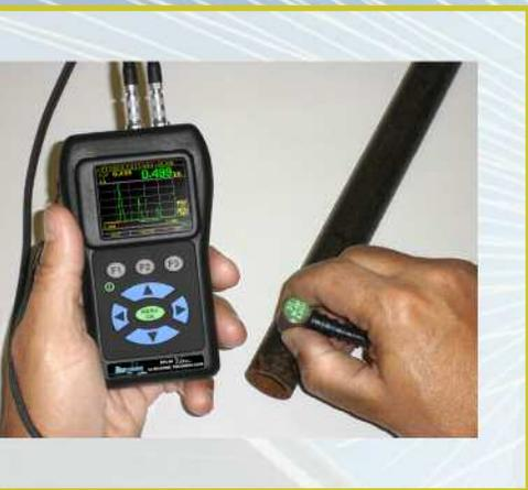
With more than 75 years of world-wide experience in Ultrasonic designs, Danatronic is proud to pioneer the world's first hand held ultrasonic thickness gage with color display; our EHC09 color wave series. Unique features include live **COLOR** A-Scan, B-Scan, 100K thickness reading (3500 waveforms) datalogger with interface program, vibration and **COLOR** change of waveform on alarm.
